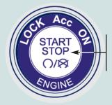
PUSH CENTER Once to change to ACC, Two times to change to ON, Three times to return to LOCK
