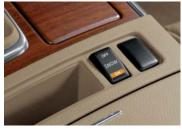
Snow Mode OFF - Push the switch to OFF for automatic AWD operation.
