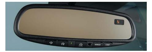
AUTOMATIC ANTI-GLARE INSIDE REAR VIEW MIRROR (with ELECTRONIC COMPASS) (if so equipped) Refer to sections 2 and 3 in your Owner's Manual.
